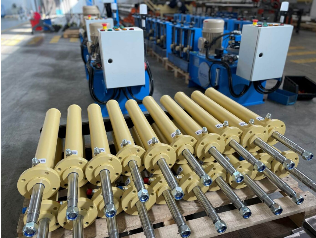
HYC-F round-flange cylinders: serial delivery batch with customer-specific painting and fittings
