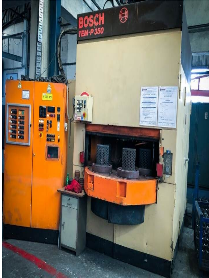
Bosch TEM-P350 thermal deburring unit — in-house burr removal for critical flow paths
